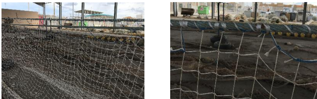
Figure 22: Polyamide trawl nettings used in the Mediterranean, here at Port-la-Nouvelle (Source: MK Développement)
