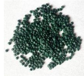
Figure 50 (opposite): rPE granules produced by Plastix in Denmark with used trawls from Brittany (Source: MK Développement)
