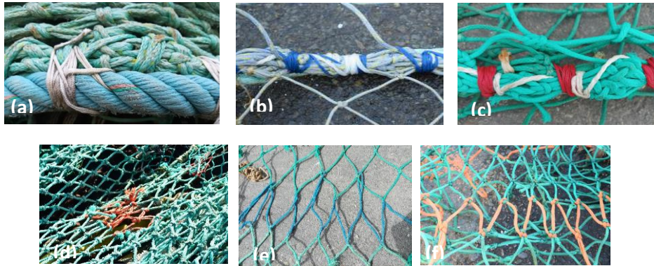
Figure 26: Various braiding and strings used to repair and mount trawls (Source: SMEL)
