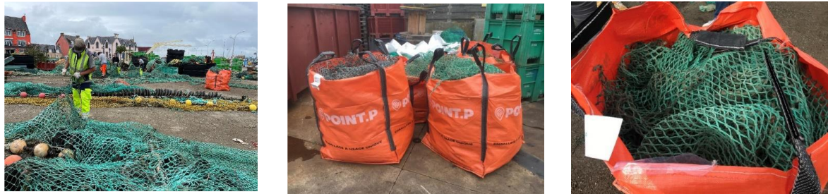
Figure 38: A used trawl dismantling operation to recycle HDPE netting (Source: FILIPECH report - port of Guilvinec)
