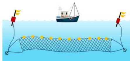
Figure 3: Set gillnet consisting of a single netting (Source: SMEL)
