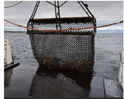
Figure 10: Brittany dredges (Source: SMEL and IFREMER)
