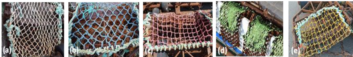
Figure 27: Plastics used in wheeled dredge netting: PA (a) and HDPE (b to e). (Source: SMEL)
