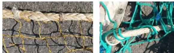
Figure 25: Dyneema rope (Source: SMEL)
