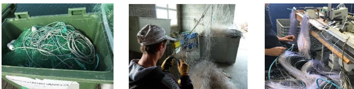
Figure 34: Used gillnet management at La Cotinière - from collection (left) to rope dismantling (centre) and re-mounting (right) (Source: PECHPROPPE report)
