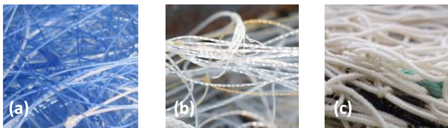
Figure 17 : Photos de filaments composant les filets : monofilament (a), multi-monofilaments (b), multifilaments (c) (Source : SMEL)
